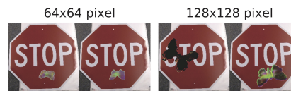
Figure 2: By placing a moth-like patch on a 'STOP' sign, we can make autonomous driving cars misrecognize the sign as 'Speed Limit 80' (Yakura et al. 2020).
